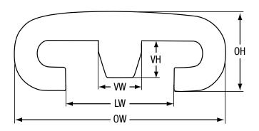
LW- Lip Width OW- Overall Width OH- Overall Height VW- Vee Width VH- Vee Height
